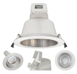
Energy efficient recessed downlight with loop-in/loop-out terminal block. Features a tri-colour selection switch to change between 3000K warm white, 4000K cool white or 5700K natural white. Ideal replacements for 4", 6" or 8" CFL downlights.
